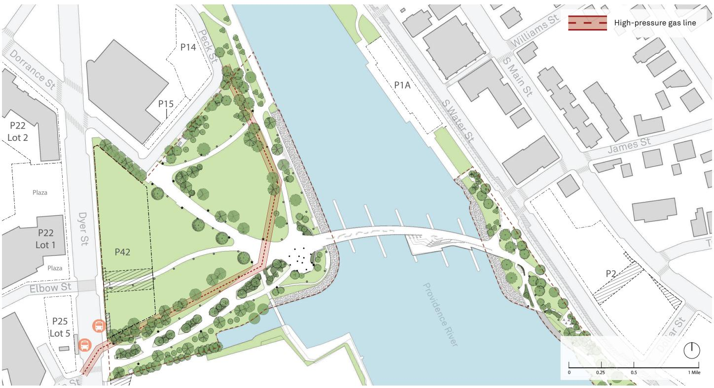
All parts of the pavilion structure and roof must be five feet away from a major high-pressure gas service line running beneath the park. Relocation of this gas line would be cost prohibitive.
